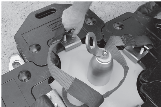
Figure 13 - Place Lifting Kit Brackets on U-Bolts
