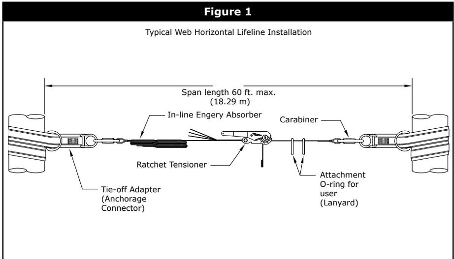
The force of striking an object in a swing fall may cause serious injury or death. Minimize swing falls by working as directly below the anchorage point as possible. Do not permit a swing fall if injury could occur. Swing falls will significantly increase the clearance required when a self retracting lifeline or other variable length connecting subsystem is used. If a swing fall situation exists in your application, contact Capital Safety before proceeding.
