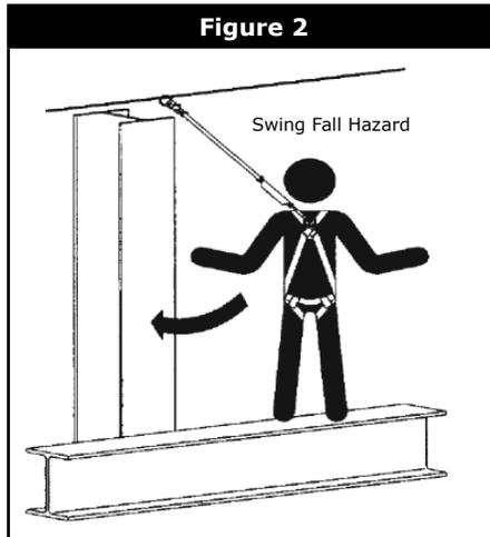
**FALL CLEARANCE:** There must be sufficient clearance below the worker to arrest a fall before striking the lower level or obstruction.
