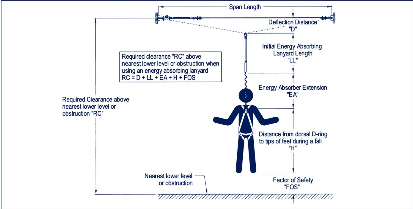
**Figure 13 - Clearance Evaluation Factors - Self Retracting Lifelines**
