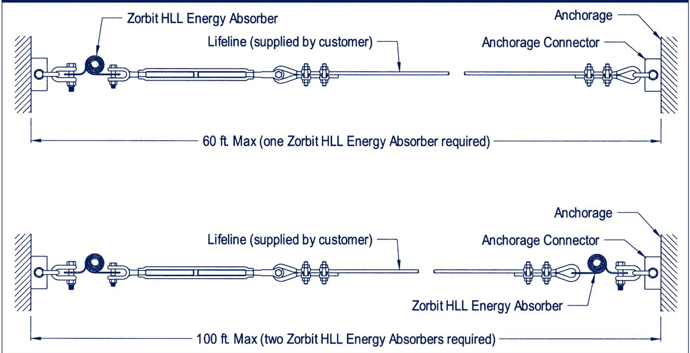
**CAUTION:** Do not rigidly mount Zorbit to structure or stanchion. May cause failure due to bending. Mount so Zorbit can pivot and move freely as shown in Figure 3.
