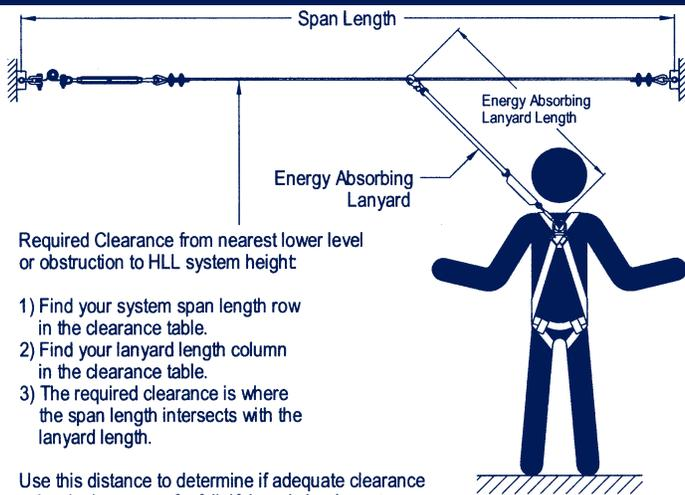
Required Clearance from nearest lower level or obstruction to HLL system height:
