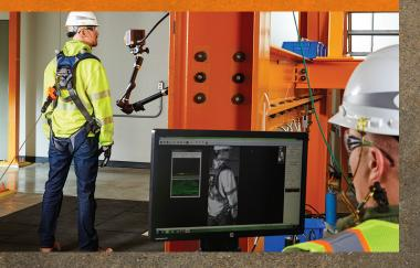
How did we create an SRL that reduces unintentional lockups? Using advanced motion capture technology, 3M studied the way users work, move and interact with SRLs on a typical job site. This data helped us engineer an arrest mechanism designed to better accommodate your natural work motions-resulting in fewer unintentional lockups.\*
